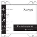
If the device is ordered with the 2Wire option, connect the two wires to the 2Wire socket. For large distances pay attention for a sufficient cable-cross-section. (For further information see [www.adatis.com](http://www.adatis.com))
