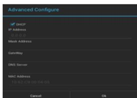
5 You can configure the IP address via the menu „advanced configure“. Select „DHCP“ for automatic mode or insert data manually.
