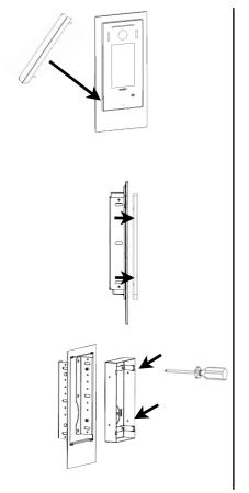
Loosen the back housing with the release tool: by pressing the release tool in the corresponding openings the front part of the device detaches.
