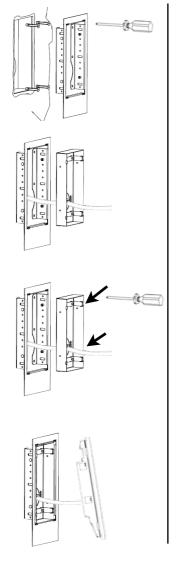
Fasten the installation frame to the wall with screws and plugs. For a clean wall finish, apply a liquid seal (e. g. silicone) around the wall cutout.
