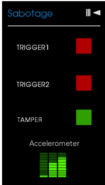
Figure 112: Configuration on the LCD display - sabotage protection
