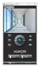
SIP client software for remote control of entrances via network, which are equipped with Adatis door terminals.
